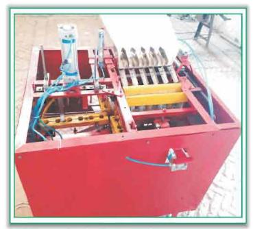
Fig 1- Pneumatic assisted coring device
