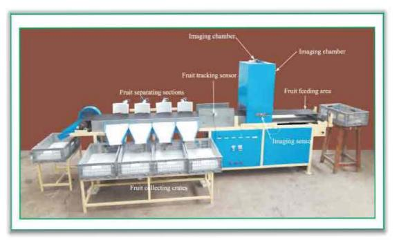
Fig 5- Automatic mango grader
